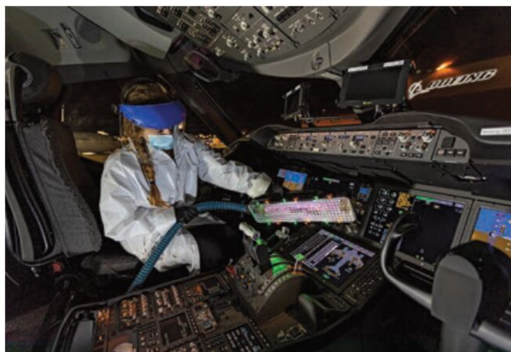
◀ A UV light wand is used to disinfect the cockpit of a Boeing plane
